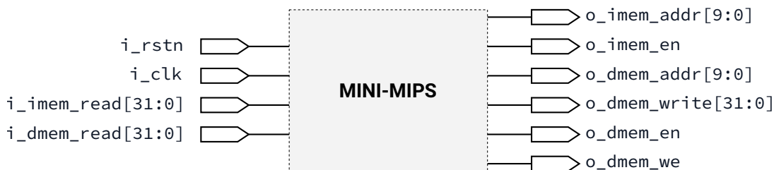
FIGURE. 10 – mini-mips ( mips_core.vhd )
