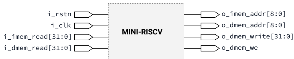
FIGURE 13: mini-riscv interface (core)
